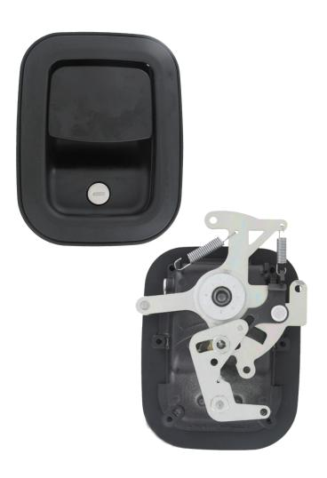
This flush mounted paddle handle with free-floating paddle (when locked) is a redesign of our popular 030-0875 Flush Mounted Paddle Handle. Containing an update to the mechanical design and with a modernized look, it can be used in FMVSS 206 (ECE R11) applications, is power lockable and features same four point pivot plate and lock cam actuation.
